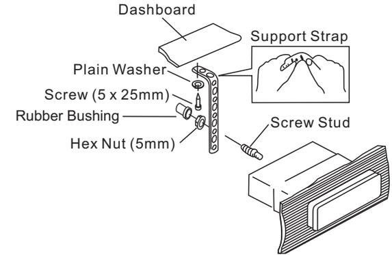
**CAUTION: The perforated rear support strap or rear rubber mounting bushing must be used in the installation of the radio. Installation without either may result in damage to the radio or the mounting surface and void the manufacturer's warranty.**
